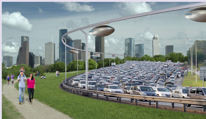
Rendering of SkyTran, an example of a PRT System that uses magnetic levitation instead of wheels.
