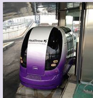
Ultra Pod PRT is a battery-powered system that operates at London Heathrow Airport.
