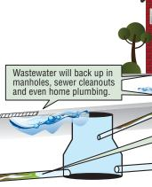
Grease and solids accumulate and block the flow of wastewater.
