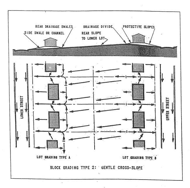
For Lot Grading Type B which drains both to the street and to the rear lot line, only side-yard swales are needed. They should extend back of the line of the rear building wall; then splash blocks from rear roof downspouts should be placed to direct roof water to the side swales for drainage directly to the abutting street. Thus the amount of water carried on the rear slope to easements or other properties is kept as small as possible. This reduces erosion and disposal problems.
